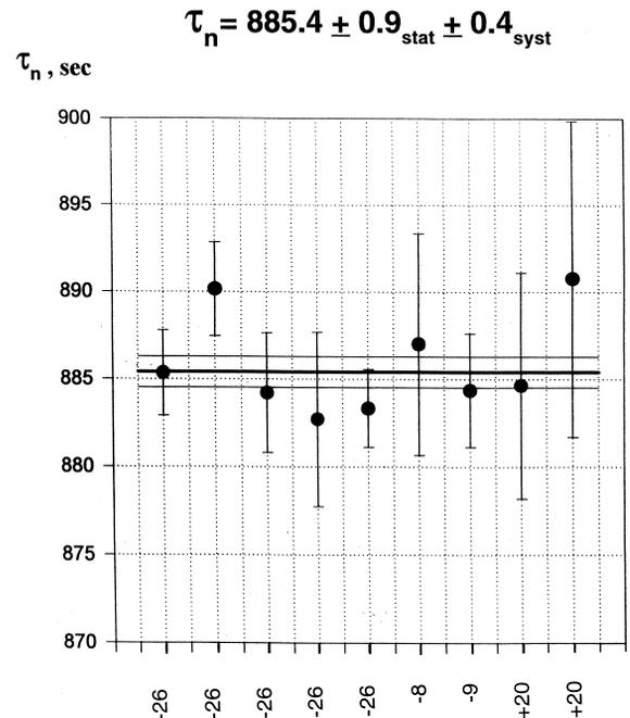
Fig. 3. Experimental values for the neutron life time from the different runs. The code for the experimental groups corresponds to the bottle temperatures  $-26^\circ\text{C}$ ,  $-9^\circ\text{C}$ ,  $-8^\circ\text{C}$  and  $+20^\circ\text{C}$ , respectively. The total measuring time summed up to 100 days.
