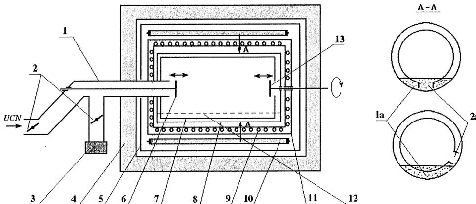
Fig. 1. The scheme of the experimental set-up. 1- UCN guide, 2- shutters, 3- UCN detector, 4-polyethylene shielding, 5- cadmium housing, 6-entrance shutter of the inner vessel, 7- inner storage vessel, 8- outer storage vessel, 9- cooling coil, 10- thermal neutron detector, 11- vacuum housing, 12- oil puddle, 13- entrance shutter of the gap vessel, 1a-oil puddle, 2a-slit.
